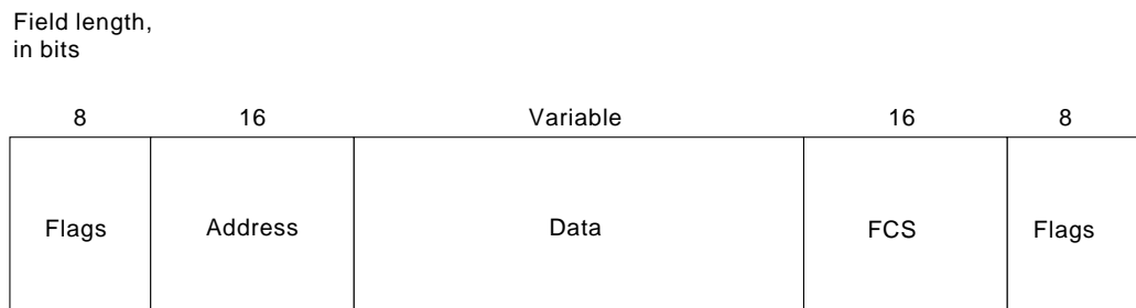
Figure 10-4 Five Fields Comprise the Frame Relay Frame
