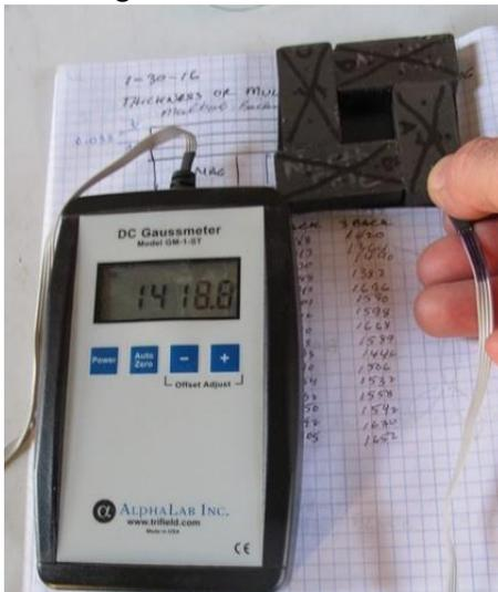
7. Place the tip of your finger over the meter probe (black probe marking up) and position the probe at each triangle center point. Disregard the negative value for the S1 and S2 magnets. Record the meter reading in your journal.
