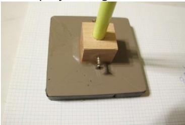
The magnets do not provide a uniform magnetic flux and vary from magnet to magnet. Use a Gauss meter to measure the strength at fifteen points on the surface of the supplied magnets. Average the measurements for all supplied magnets.
