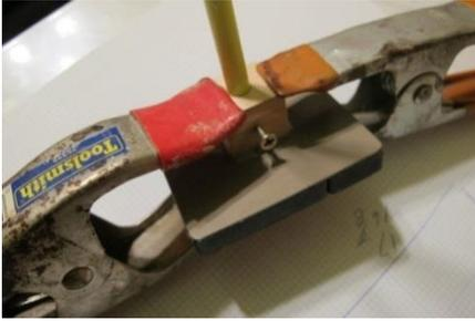
14. Remove the shaft after a few minutes while not disturbing the clamps.
