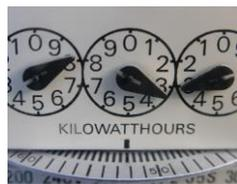
If power is measured in **watts** and **multiplied** by the **hours** of use, the resultant is **watt-hours (Wh)**.
