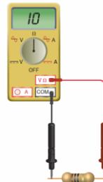
**Ohmmeters should never be connected to live circuits!**
