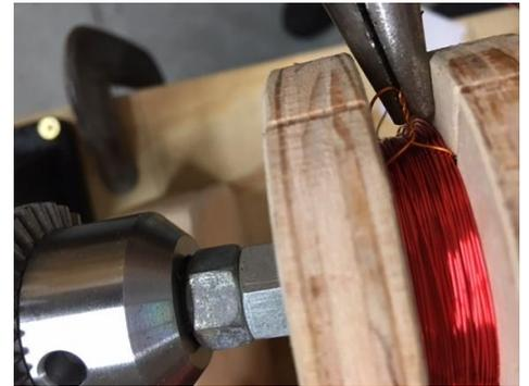
Twist the ends of the coil-holding wires
