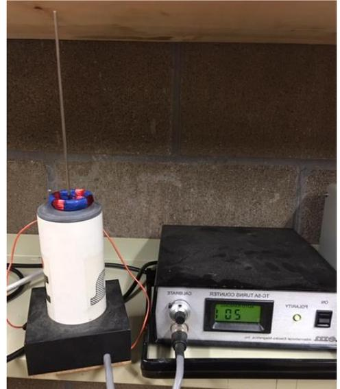
14. Measure the inner and outer diameters and the thickness of the each coil in mm. Use the supplied digital calipers for the measurements. Each team member should perform three the measurements for diameters and thickness on a coil and average the data. In other words, one member measures coil-A then another coil-B and so forth.
