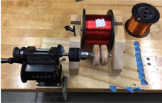
Coil Winding Setup
