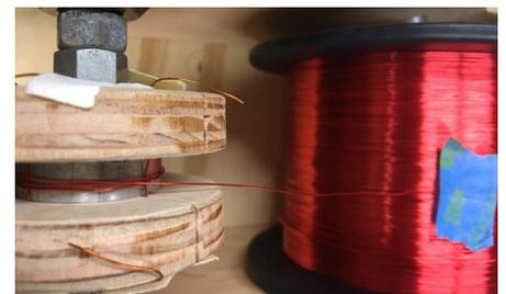
5. Hand wrap three turns around the core while applying tension to the wire spool.
